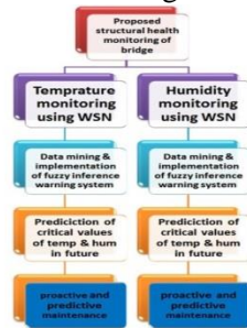
Figure 1. An overview of proposed SHM system and its components and function.
