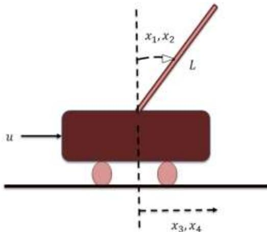
Figure 3. The inverted pendulum on a movable cart.
