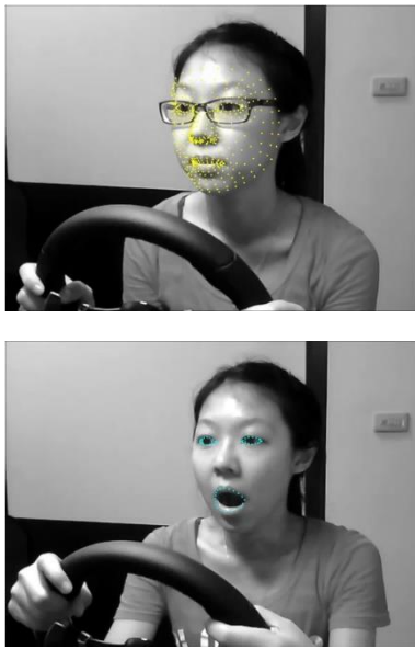
Figure 2. Face and keypoint detection on one frame: a) 468 points, b) Selected 52 points.
