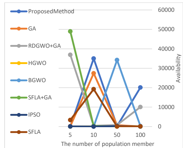
Figure 23. Availability of the SN (AQV) by the selection methods when the number of web services is 100 and initial population increases.
