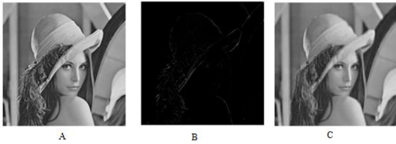
Figure 2. Decomposition of a gray image based on PCA, (A) Original image (B) Image of sparse component (structure), (C) Image of low rank component (texture).
