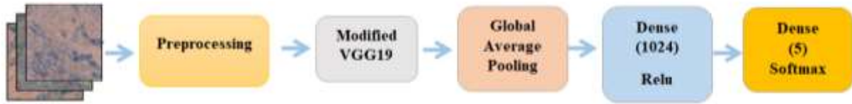
Figure 1. Flowchart of our Proposed Method for Direct Fungal Infection Detection Using modified VGG19.
