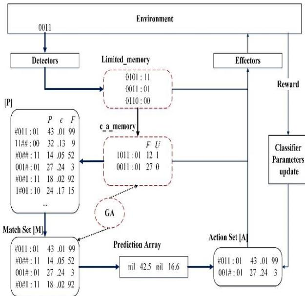
Figure 1. Proposed architecture for an LCS.
