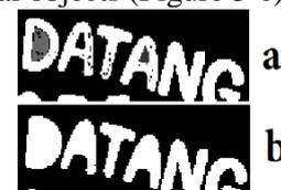
Figure 6. (a) Small holes near edges (b) Filled MSER regions.
