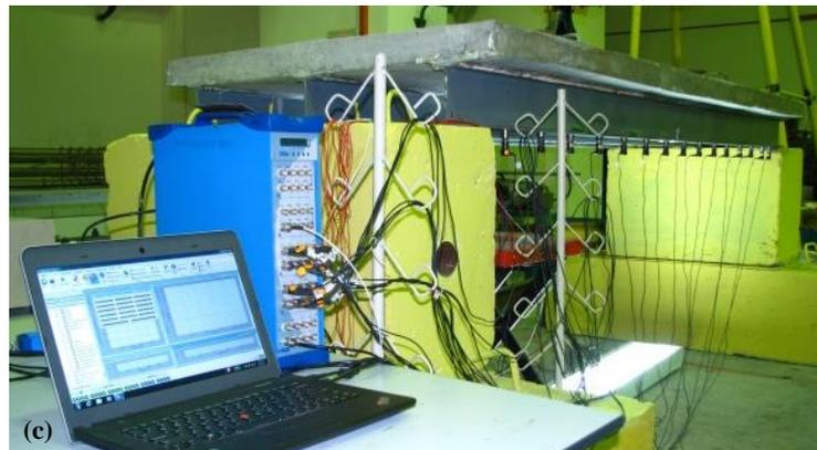
**Figure 2. Experimental work: (a) layout plan of the composite bridge, (b) drawing of the experimental setup, and (c) physical observation of the vibration test.**
