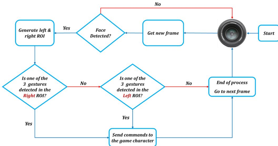
Figure 4. A flowchart for the hand gesture recognition using a multi-class classifier.
