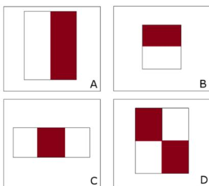
Figure 2. Four sets of rectangles in the Haar-like feature extraction.
