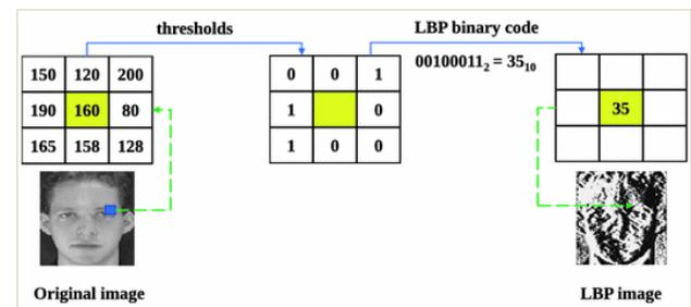
Figure 1. Algorithm of the local binary pattern.
