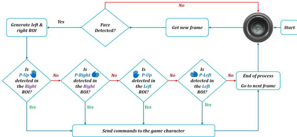
Figure 5. The proposed flowchart for the hand gesture recognition using single-class classifiers for hand gestures.
