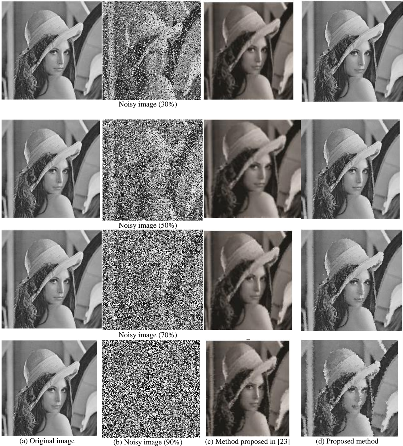
Figure 4. Comparison results of the proposed method with the one proposed in [23] for Lena image on different noise rates.
