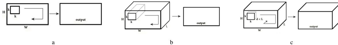
**Figure 3. Graphical illustration of the effects of 2D and 3D convolutions on 2D (images) and 3D (videos) input data. a) 2D input and 2D convolution b) 3D input and 2D convolution c) 3D input and 3D convolution [21]. W, H, and L are width, height and length (number of frames) of the input data, respectively. Size of the 2D Convolutional filter is  $k \times k$  and the 3D filter is of size  $k \times k \times d$ , where  $d$  corresponds to the depth of the filter.**
