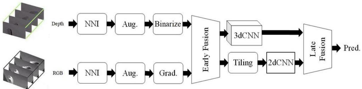
**Figure 1. Block diagram of the proposed method. Input is the RGB and depth modalities of hand gesture videos, and the output is the predicted label. The following modules are used in the framework. NNI: Nearest Neighbor Interpolation, to fix video lengths; Aug: Data Augmentation. Binarize layer generates a binary image from depth data. Grad. Layer calculates Gradient from intensity channel of color data using Canny operator, Tiling, generates a 2D pattern from sequence of video**
