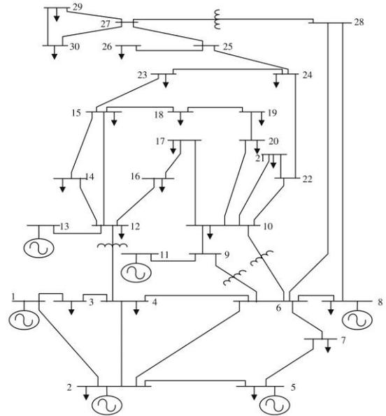
Figure 3. IEEE 30-bus test system
