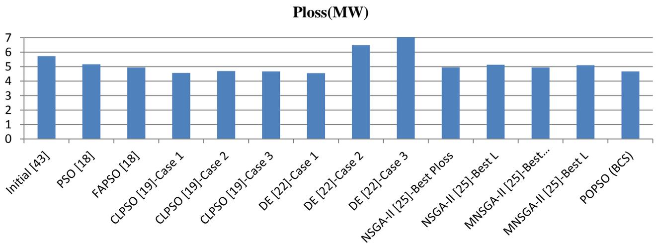
**Figure 9. Comparison results of power loss in IEEE 30-bus test system**
