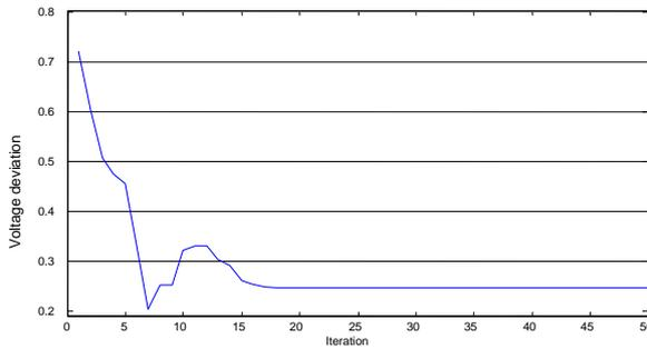
Figure 6. Convergence of best compromise solution voltage deviation
