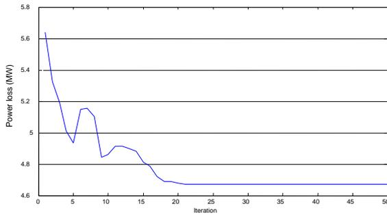
Figure 5. Convergence of best compromise solution power loss
