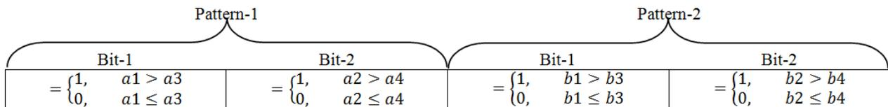
Figure 3. Single pixel representation using two separate patterns
