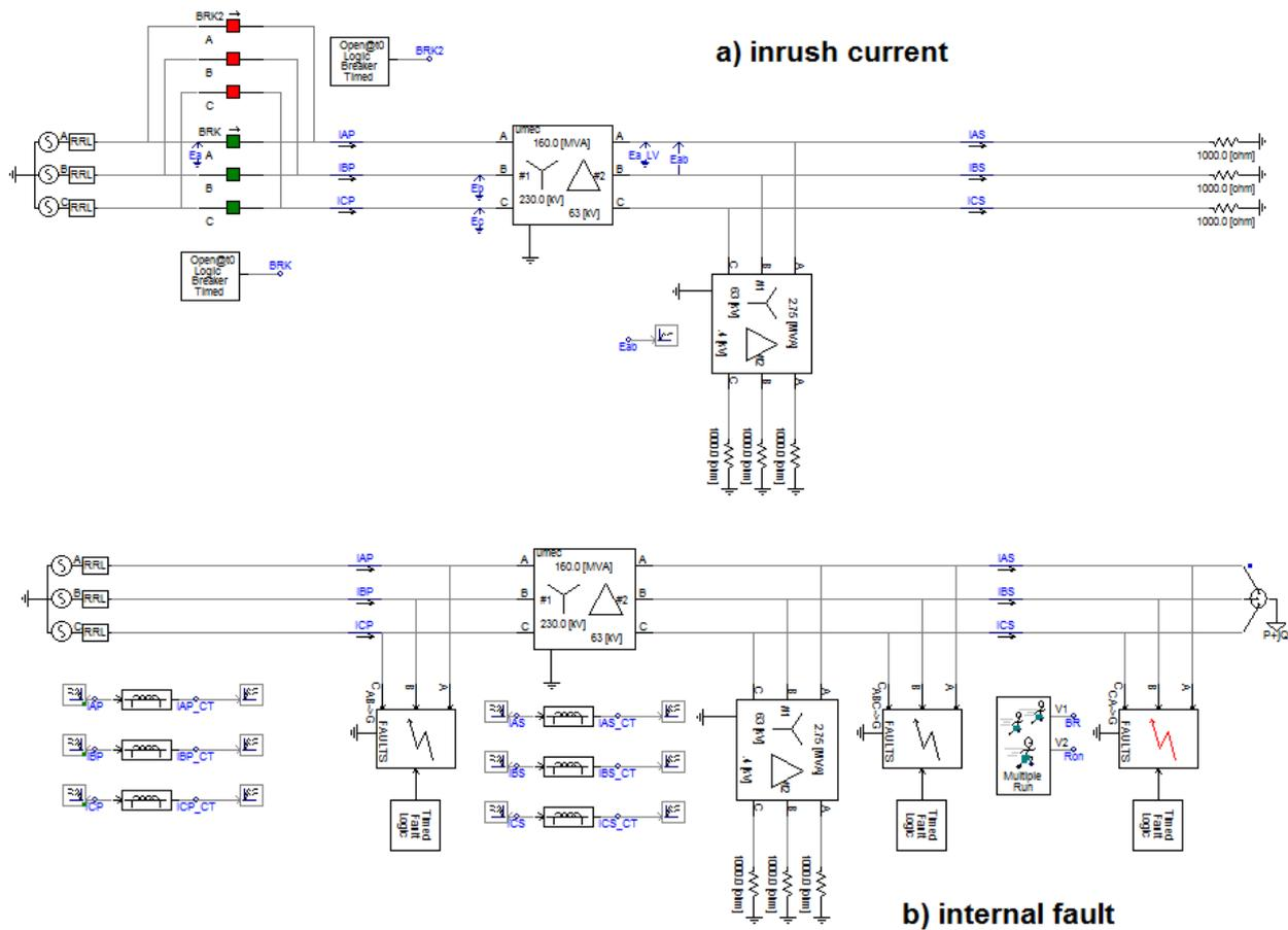
Figure 6. View of power system model, a) model of inrush current, b) model of internal fault current.
