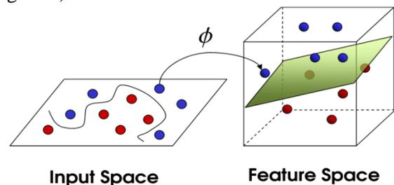
Figure 4. Concept of non-linear kernel function
