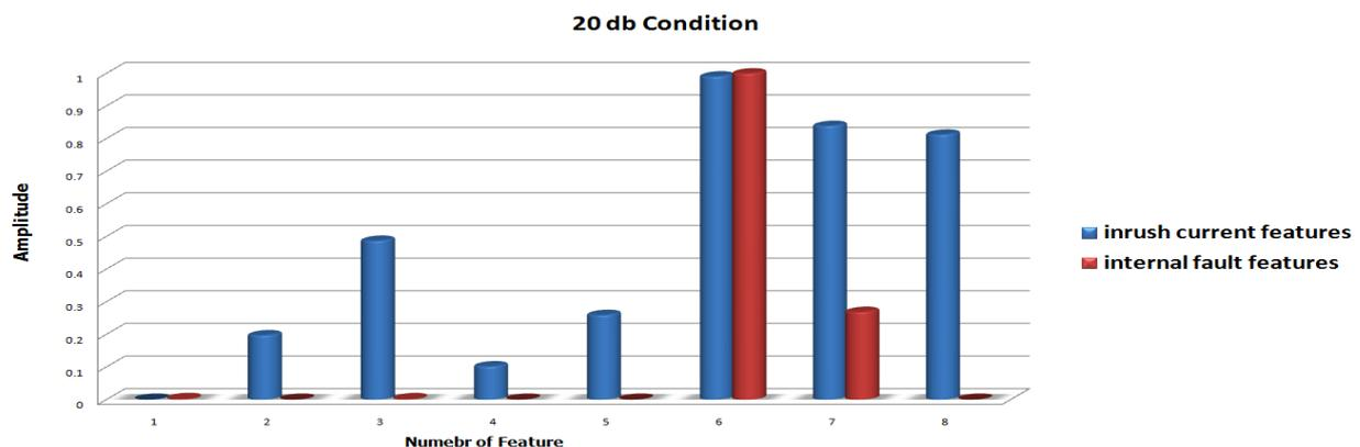
**Figure 3. The values of the features of inrush current and internal fault in 20 dB noise condition.**
