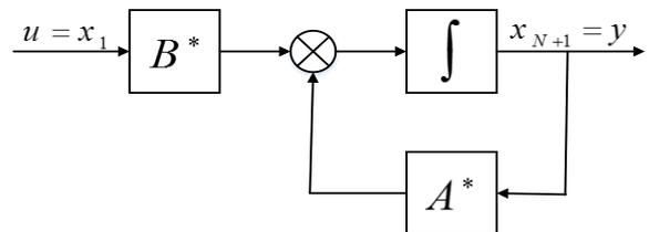
Figure 2. State-space representation of operator [19].
