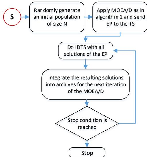
Figure 2. Flow chart of proposed algorithm (MOEA/D-TS).
