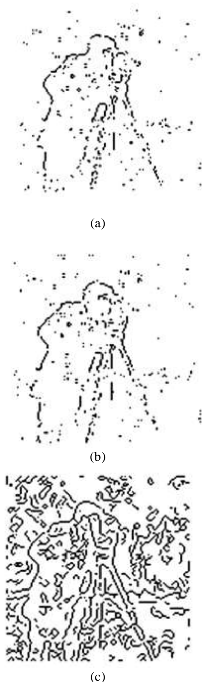
Figure 4. edge detection with salt and pepper noise and intensity= 0.1 (a) edge detection with Sobel operator, (b) edge detection with Prewitt operator, (c) edge detection with Canny operator.
