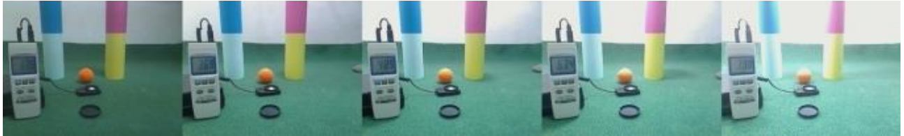
Figure 4. Five samples of increasing illumination recorded by lux meter.
