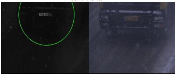
Figure 10. Detection of vehicle in snow conditions.
