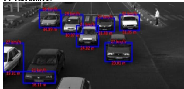
Figure 7. Vehicle speed tracking.
