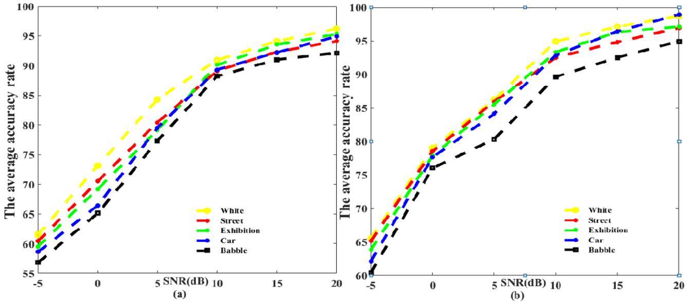
Figure 8. Evaluation of proposed method in comparison to previous technique for speech/silence detection. (a): Combination of auto-correlation function, ZCR, and cepstral peak. (b): Proposed method using GMM clustering.
