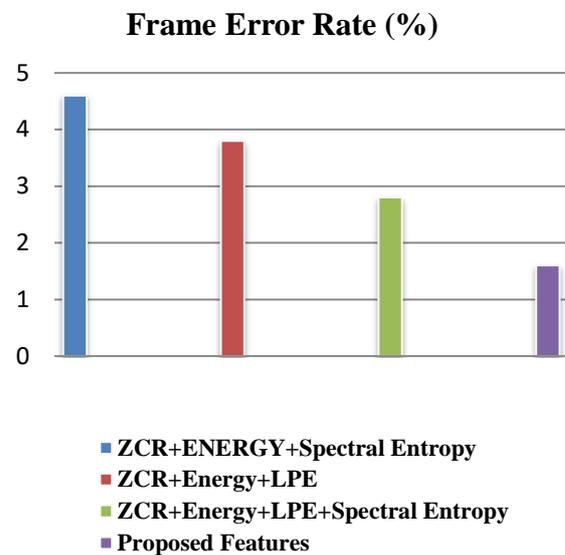
**Figure 6. Frame error rate of proposed features in comparison to conventional features.**
