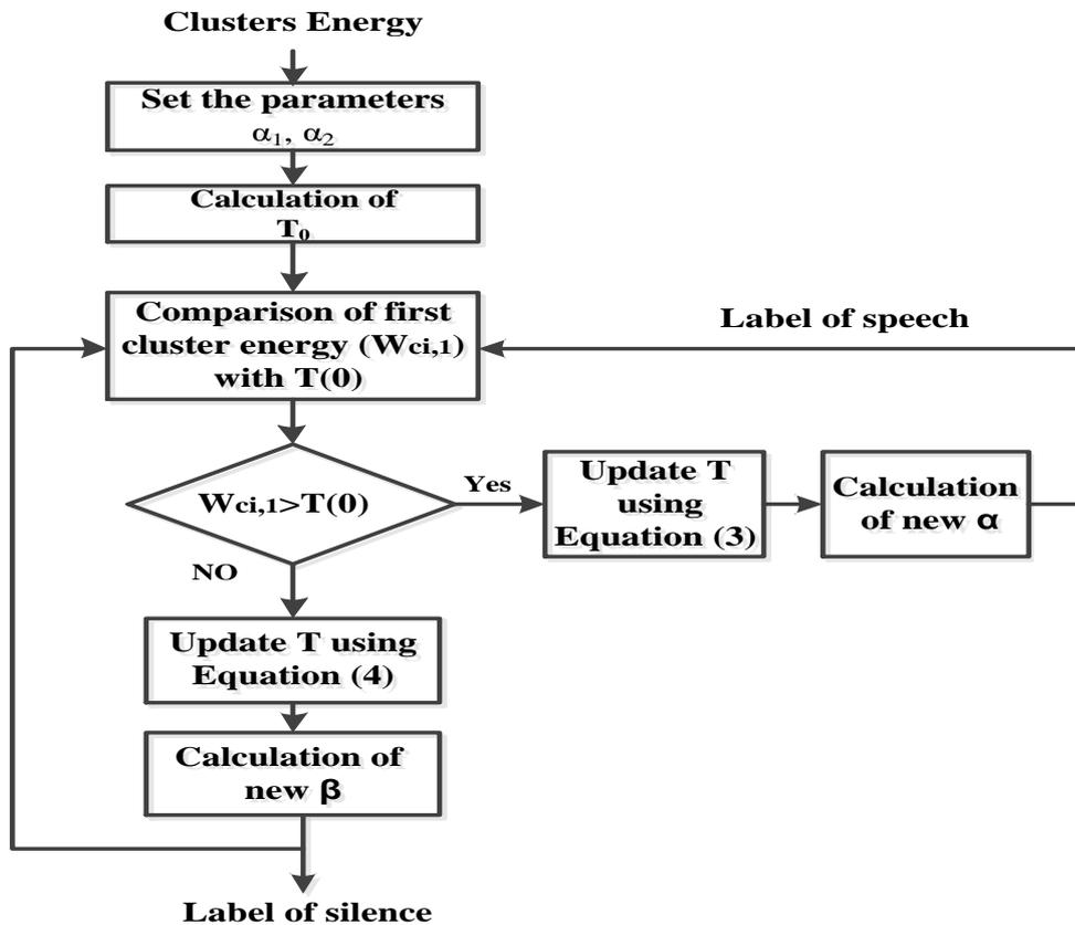
Figure 2. A flowchart of proposed method for silence/speech detection..
