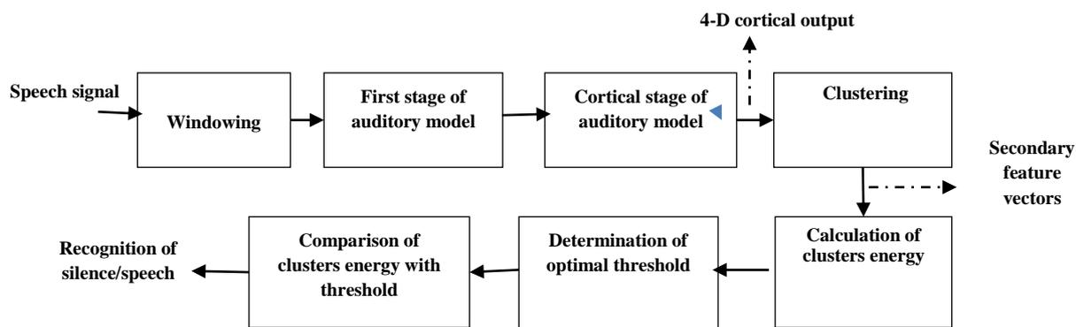
Figure 1. Block diagram of proposed method for silence/speech detection.
