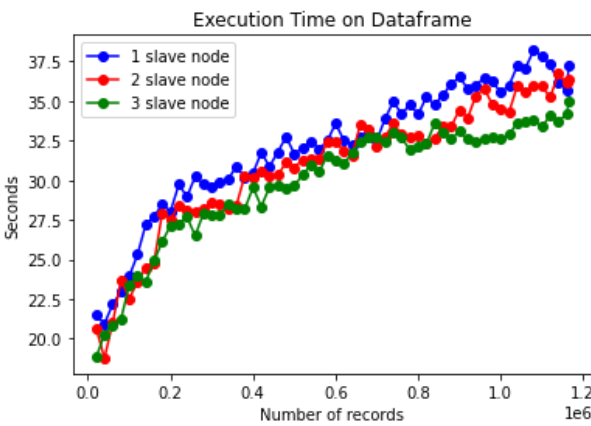
Figure 5. Evaluation of proposed framework based on different number of slave nodes (million records).
