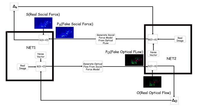
Figure 3. Generator of first network (left) generates an optical flow image from social force, and generator of second network (right) produces a social force image from optical flow.
