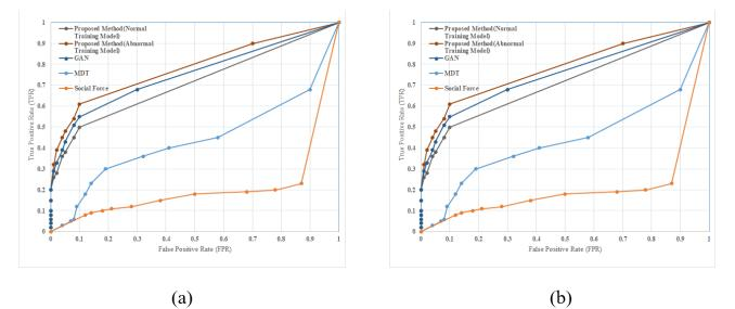
Figure 4. Comparison of abnormal behavior detection methods using ROC curve in UCSD database. a) ROC curve in framelevel b) ROC curve in pixel-level.
