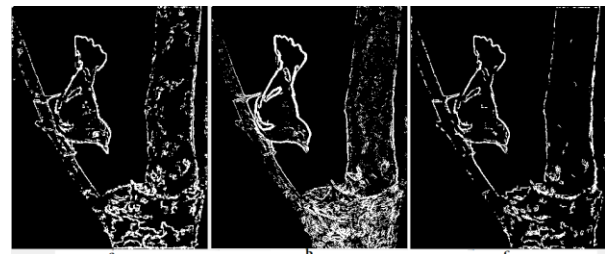
Figure 9. (a) The binary mask. (b) result of Otsu method. (c) a multiplied by b.
