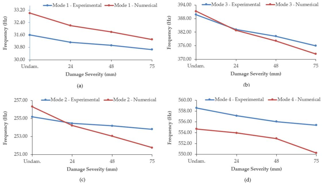
Figure 7. Evaluation of the experimental and finite element simulation findings in the (a) 1<sup>st</sup> mode, (b) 2<sup>nd</sup> mode, (c) 3<sup>rd</sup> mode, and (d) 4<sup>th</sup> mode .
