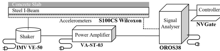
Figure 3. Illustration of the experimental modal analysis.
