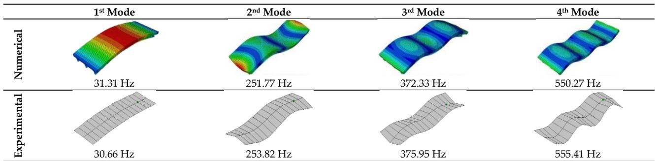
Figure 6. Experimental and numerical first four mode shapes.
