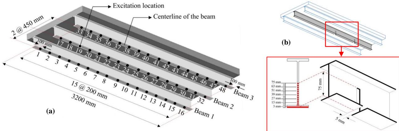
Figure 4. (a) Positions of accelerometers and shaker, and (b) conducted damage cases.
