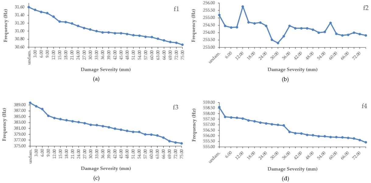
Figure 5. Natural frequencies of intact and damaged structure in the 1<sup>st</sup> four modes: (a) f1, (b) f2, (c) f3, and (d) f4.
