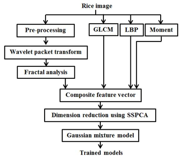
Figure 5. A block diagram of the proposed rice classification algorithm.
