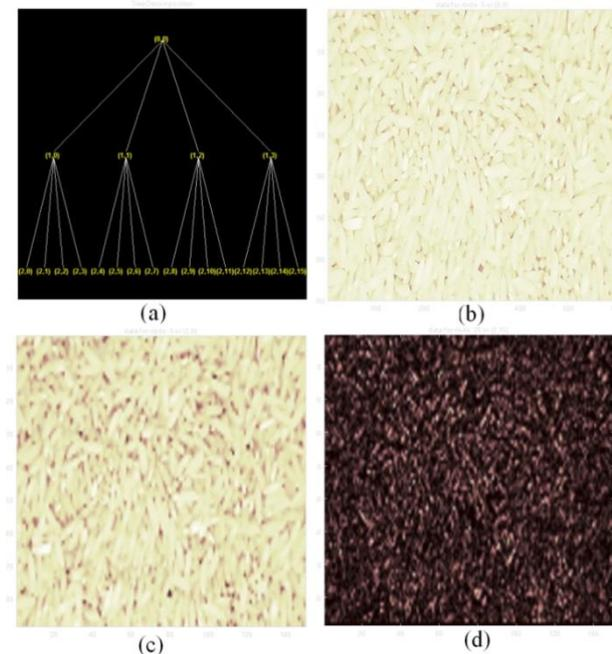
Figure 4. a) Wavelet packet transform tree with decomposition level 2. b) Bulk sample of Hashemi rice in the node  $(0, 0)$  of the analysis tree. c) Transformed image in the first sub-band of decomposition level 2 (node  $(2, 0)$ ). d) Transformed image in the last sub-band of decomposition level 2 (node  $(2, 15)$ ).
