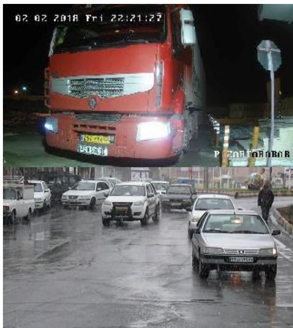
Figure 3. Some IRVD images suitable (bottom) and not suitable (top) for license plate recognition.
