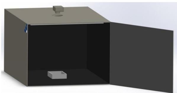
Figure 2. Box designed to record image of the rice grains.
