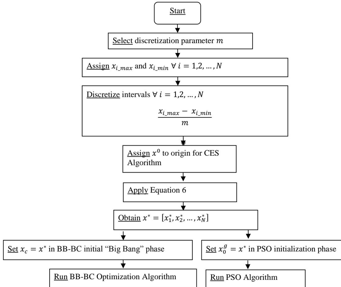
Figure 2. The flowchart of CES-BB-BC optimization and CES-PSO algorithms.
