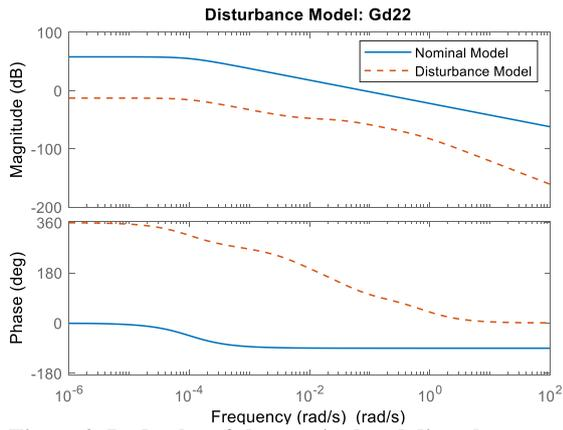
Figure 9. Bode plot of the nominal and disturbance model.
