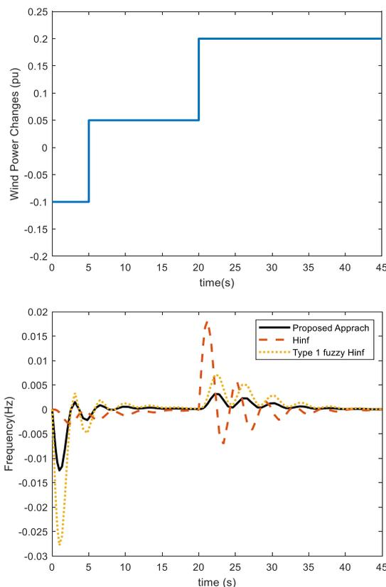
Figure 16. Comparison of the controller against wind power changes.
