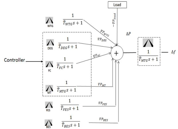
Figure 2. Proposed interval Type II fuzzy dynamical model.
