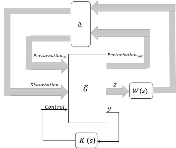
Figure 7. LFT framework of the proposed structure.
