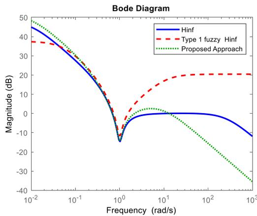
Figure 15. Comparison of alternative controllers.
