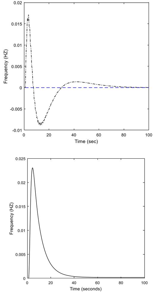
Figure 14. Closed Loop Time Response (top) and disturbance rejection (bottom).
