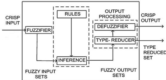
Figure 1. Block diagram of IT2FLC.
