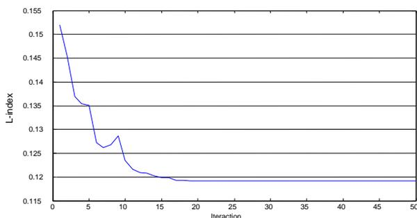
Figure 7. Convergence of best compromise solution voltage stability index
