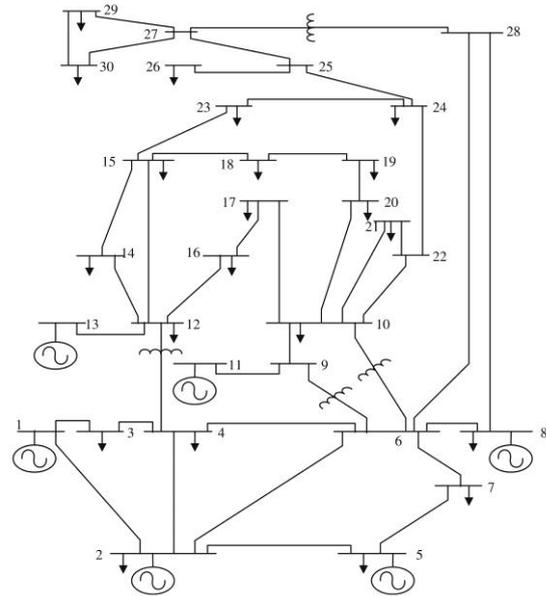
Figure 3. IEEE 30-bus test system
