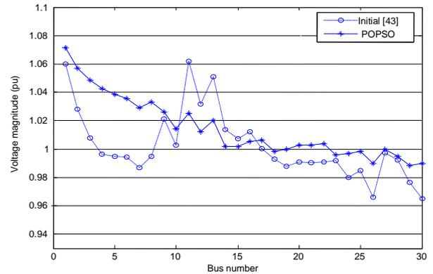
Figure 8. Bus voltage profiles
