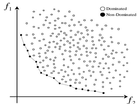
Figure 1. Depiction of domination using a two-objective minimization case
