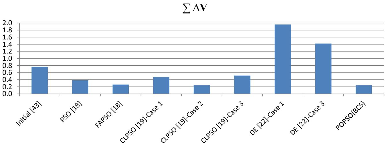
**Figure 10. Comparison results of voltage deviation in IEEE 30-bus test system**
