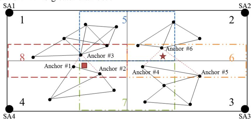
Figure 4. Localization of nodes ★ and ■ after segmentation of field to four non-overlapping and four overlapping sub-regions.
