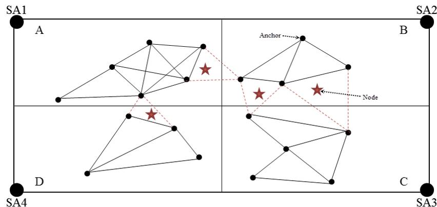
Figure 3. Non-formation of triangles because of residence of anchors in different sub-regions.
