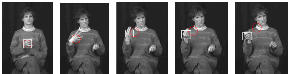
Figure 7. Hand tracking for the usual image by applying the combination of mean shift and motion detection algorithms.
