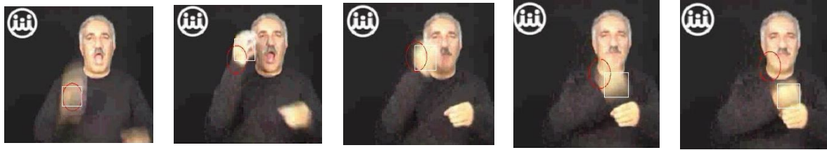
Figure 8. Hand tracking for complicated image by applying mean shift and motion detection algorithms.
