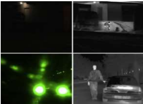
Fig. 1. Visible images (left column) and thermal images (right column) of the same scenes that pedestrians are detected in thermal images with insufficient or over illumination [4].
