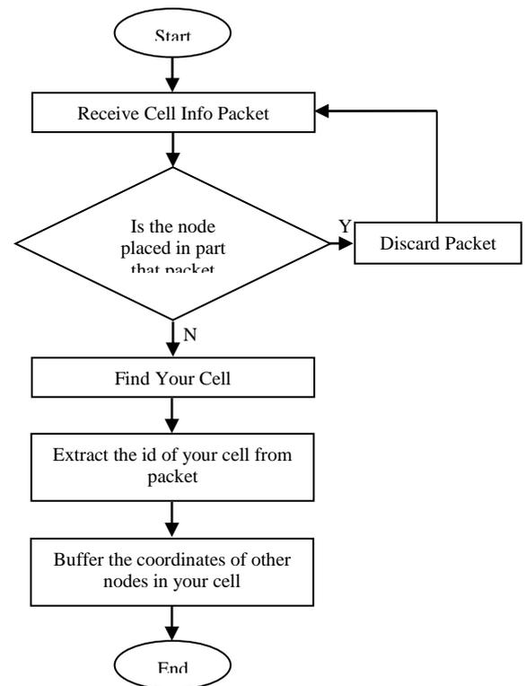
Figure 4. Finding cell and other nodes in cell.
