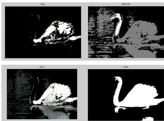
Figure 3. Segmentation results obtained from SNN (Left-top), DBSCAN (Right-top), GMM (Left-down), and WMM (Right-down).
