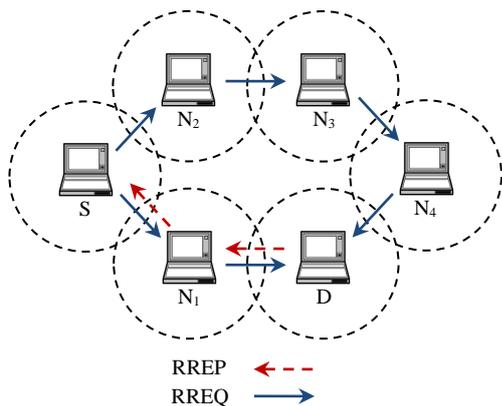
Figure 1. Routing process in AODV protocol
